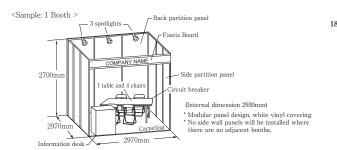
One booth is approximately 9.0 sqm (2.97 m (W) x 2.97 m (D) x 2.7 m(H)) of floor space. Multiple booths are aligned in single or double rows
